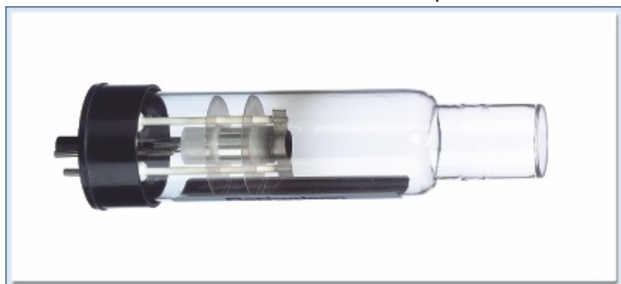
37 mm standard hollow cathode lamp
