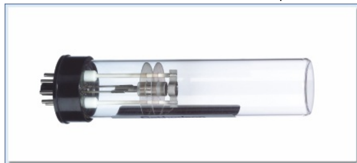
50 mm hollow cathode lamp (Perkin Elmer AAnalyst coded)
